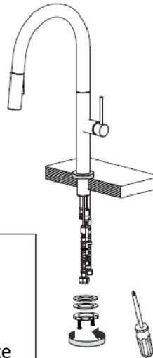
**3** On the handspray side of the hose, measure 15" down from the body of the faucet and make a mark. Install the hose weight at the mark. Reposition the hose weight as necessary to insure the handspray pulls out and retracts smoothly.
