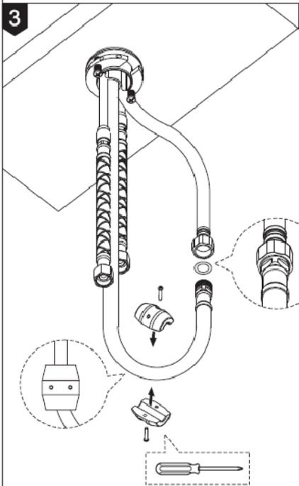
Make sure that the supply hoses do not interfere with the pullout hose. If necessary, reposition the hoses.
